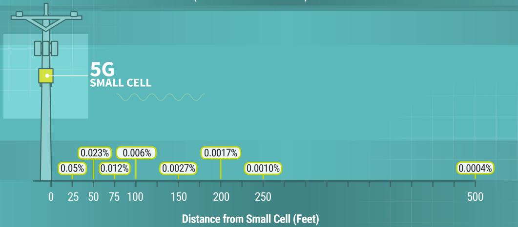
This chart shows typical exposures as a percent of the FCC limit for a 5G small cell. The limit is generally taken to be a worst case (whole body) exposure value from a source whereas a typical exposure is a more realistic exposure one might expect to receive from a given source. The maximum exposure would usually exist only at a specified distance from the source whereas the typical exposure might occur at a wide range of locations and represent a more realistic exposure from a given source.
