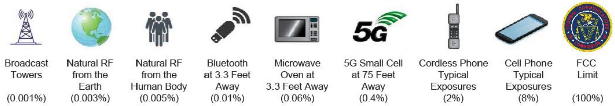
Figure 2. Ranking of common examples of RF sources by percent of FCC limit from left (lowest) to right (highest).
